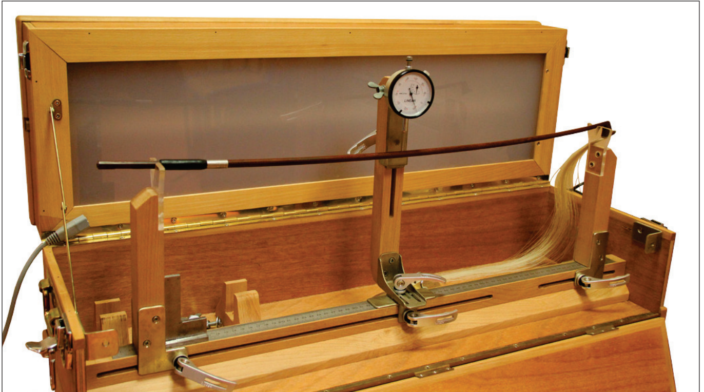
Figure 4. Bow characterization device prototype (PAFI project): mechanical and geometrical parameters measurements.
