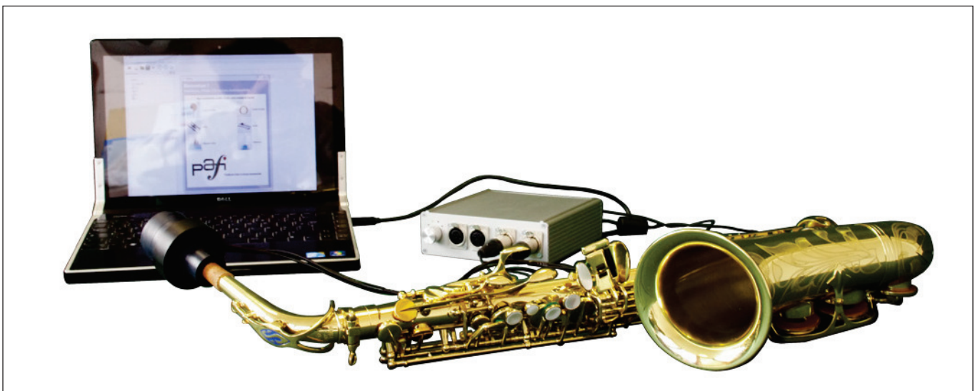
Figure 5. Wind instrument device prototype (PAFI project): input impedance measurement. The input impedance, measured or calculated, is a quantity that gives important information regarding instrument playing behaviour. It characterizes air column resonances from a given bore geometry (see [13], [14], [15], [16]).
